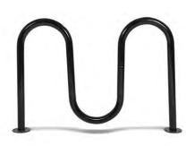
W: 50 1/2" D: 2 3/8" H: 34 1/4" Rack Material: 2 3/8" tubing Mounting Options: In-ground or surface-mount Finish Options: Powder-coat (see pages 116-117) Rack Dimensions: 4' 2" length - 5 bikes
